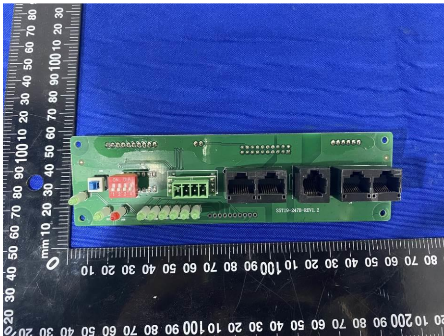
Figure 12 Front view of PCB for communication
